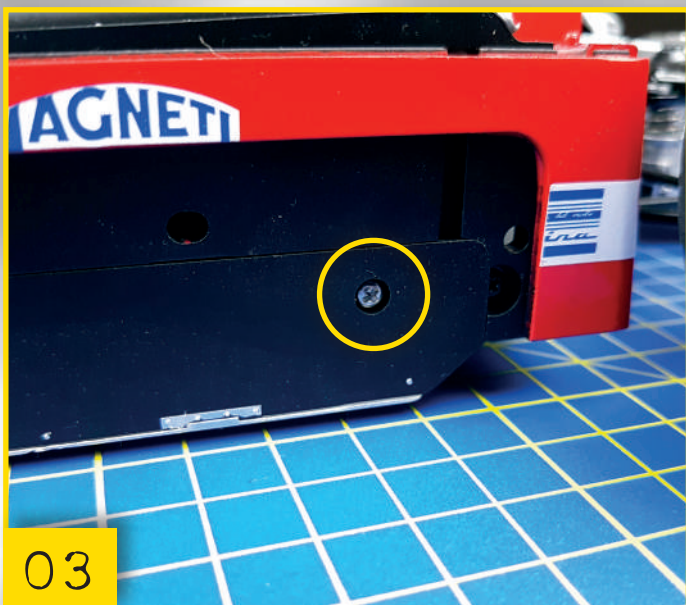
93-03 Insert and tighten a type P screw in the first hole (A) in the front.
