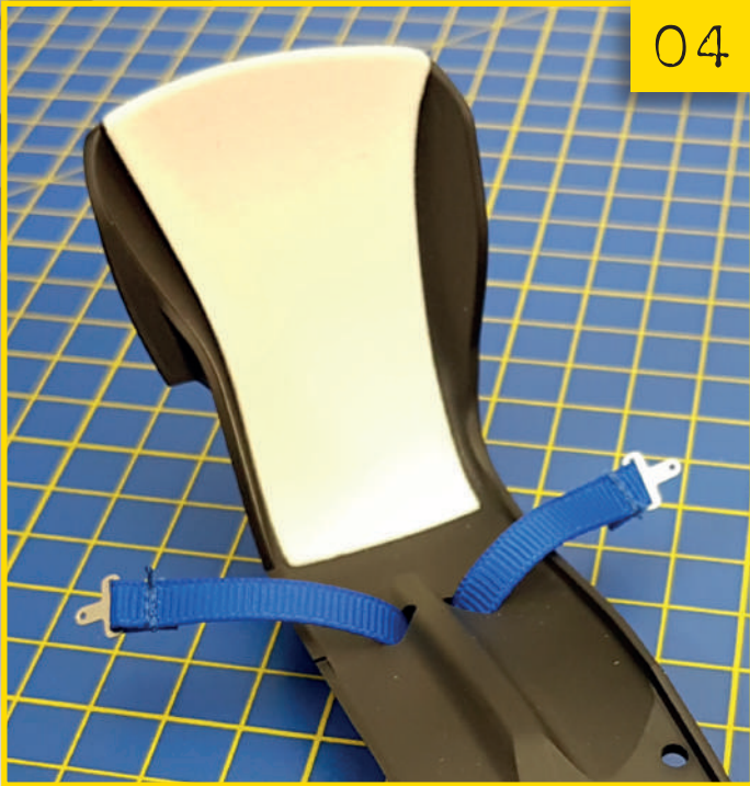
50-04 Take the seat and pass the seatbelt through its openings, as shown in the image.
