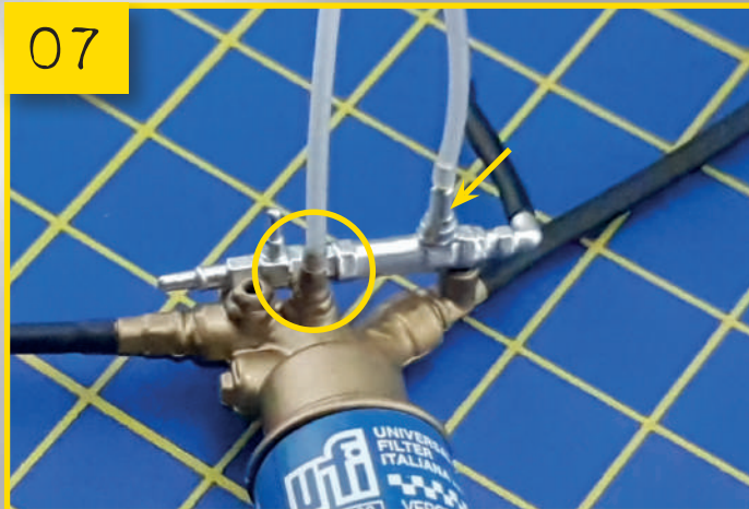
18-07 Join the two white pipes to the fuel line connector. The small circle in the photo shows the connection for the short pipe, the arrow shows the connection point for the longer pipe.
