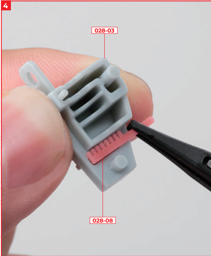
Insert the leg position pointer 028-08 into the shaft retainer 028-03 .
