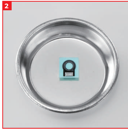
Float the decal 027-03 in the dish of water with the printed side facing up and wait for about 10 seconds.
