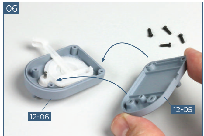
Fit the other half of the gearbox housing 12-05 over part 12-06 as indicated.
