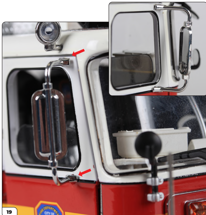
Fix the right-hand wing mirror in place, pressing it firmly into the two fixing points indicated above.
