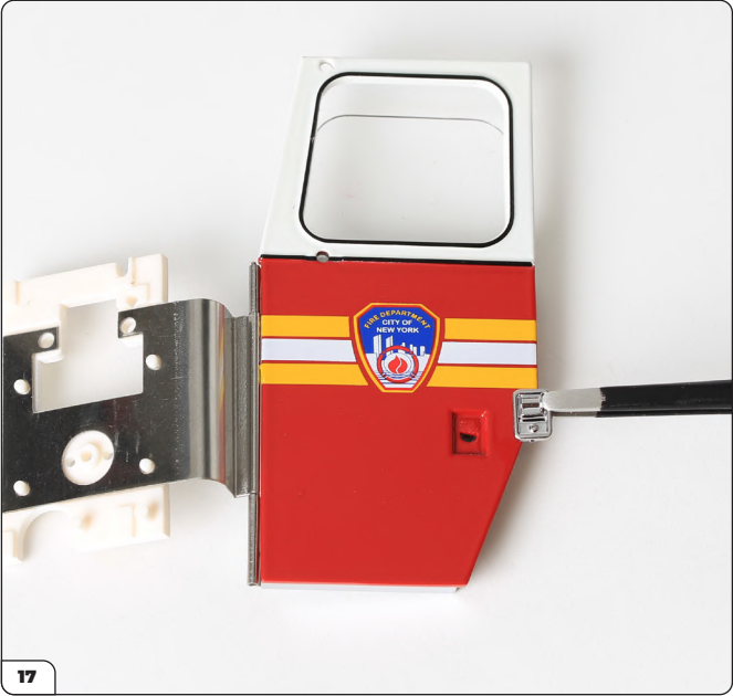
Press the handle into position. This is a D-shaped fitting to ensure the correct fit.
