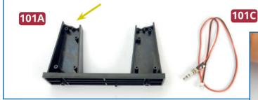
Position the metal terminal of the cable C (101C) in the recess in the upright part of support 101A. Note that the terminal is fitted in the side of the support indicated by the arrow (above). The neck of the terminal is gripped in the support (below). Then pass the plastic plug on the other end of the cable through the hole at the base of the support (below right).
