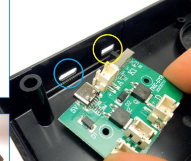
Turn the battery box **104A** upside down and check how the circuit board **104B** fits: screw holes on part **104B** align with sockets on the battery box (circled in white, above left). As you position the circuit board, the switch fits into one slot (circled in yellow) and the USB port fits into the adjacent slot (circled in blue).
