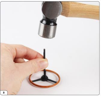
Carefully hammer the steering column into the steering wheel.
