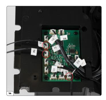
Plug wires '12', '13' and '14' into the corresponding sockets.
