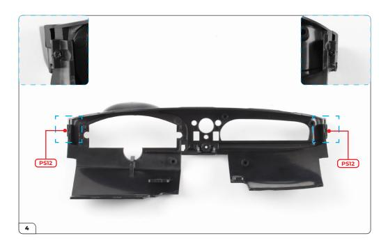
Use 2x PS12 screws to secure in place.
