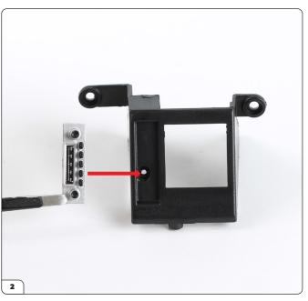
Fit the radio into the GPS housing (55-A).
