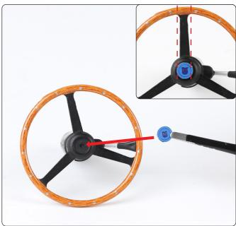
The flat end of the steering column align with the top spoke of the wheel (left image). Align the steering wheel badge (57-E) with the steering wheel then press into the recess. The badge should align with the top spoke (inset).
