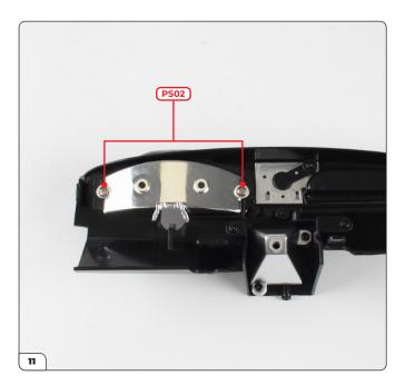
Fit the reflector onto the screw posts then fix in place with 2x PS02 screws.
