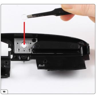
Place the clock lens (54-E) into the hole.
