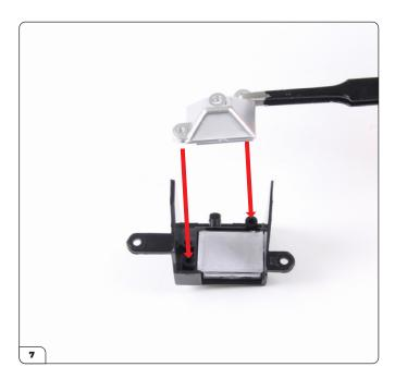
Align the GPS reflector (55-E) with the screw holes on the housing.
