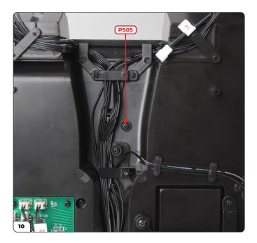
Secure the GPS housing to the cockpit by driving a PS05 screw into it from underneath.
