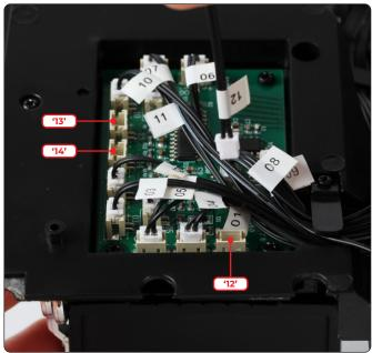
Next you'll connect the remaining wires to the circuit board. Sockets 12, 13 and 14 have been highlighted in the images.
