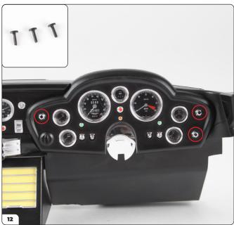
The three switches (56-G, inset) fit into the holes in the housing (circled).
