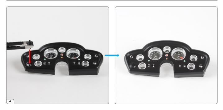
Fit the air vent switch (56-F) into the shaped hole in the housing.
