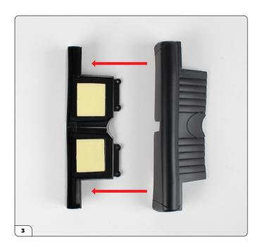
Align the rear seat cover (51-B) with the base.
