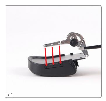
Align the passenger backrest adjuster ("L1") with the three holes on the side of the backrest.
