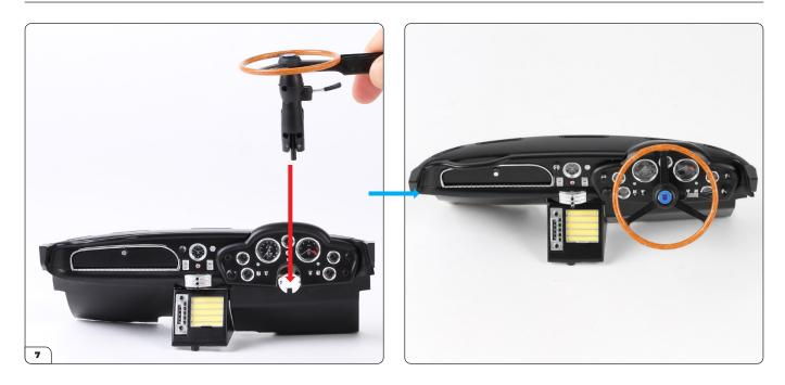
Fit the steering wheel cover into the dashboard (stage 056). The hole is shaped to ensure the correct orientation.
