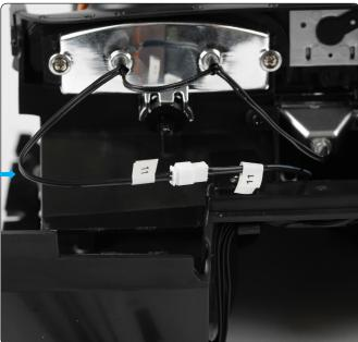
The bulbs should look like this once fitted. Connect the two wires marked '11' together.
