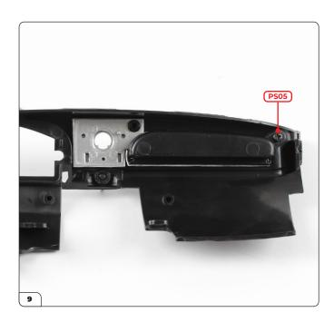
Fit the glovebox in place and secure with a PS05 screw.
