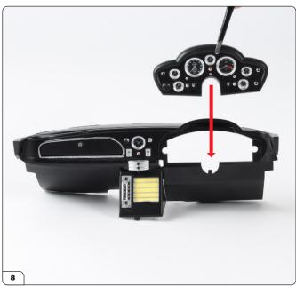
Align the housing with the dashboard (stage 055) as shown.
