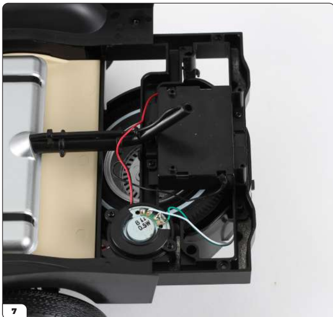
Before fitting the circuit board, ensure the black and red wires are moved away from the battery compartment as shown.
