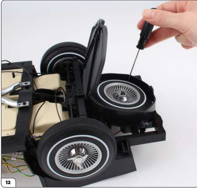
Using a screwdriver or similar tool, lift the spare wheel out of the holder and place it aside.
